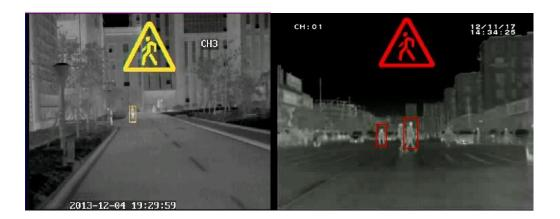
2) When pedestrians walking in front of the driving vehicle with the distance of 40m to 90m, the pedestrians will be marked with a rectangular box in yellow, at the meantime, the display will shows a yellow triangle icon to pre-alarm when pedestrians approaching; meanwhile the PSD NV will eject a yellow triangle icon on display and blares in one alarming sound to pre-alarm.
